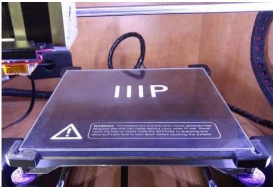
Fig 4: Build platform with a manual levelling mechanism
